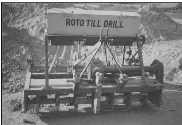
Fig. 5.12 : Roto Till Drill - A modern agricultural equipment
